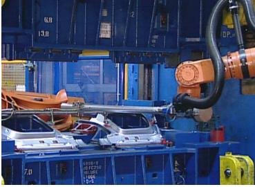
Robotic automation between tandem presses may not be the fastest solution, however for certain applications they provide the flexibility required. These applications may include an extremely large or heavy blank, the need for precise placement in the press or the requirement to turn a blank over.
