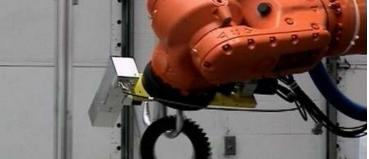
**Imagine** ... A robot poised in the pounce position while a part is exiting a machine on a run out conveyor. As the part draws near the robot, a series of cameras photograph the part and send the position data to the robot controller. The robot picks the part up and precisely places it into a container in a matter of seconds.
