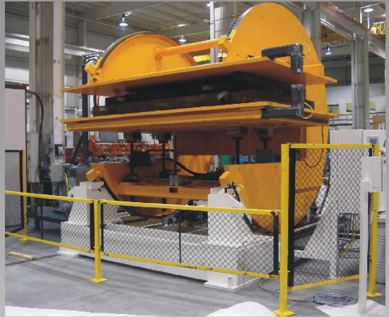
The Atlas "C-Frame" Bundle Turnover handles parts by entering in one side, turning over, and exiting out the other end with a fork truck.
