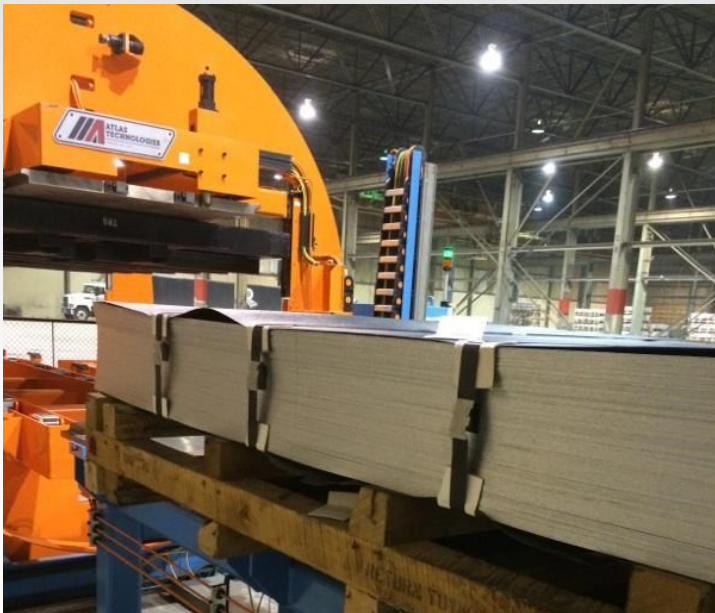
Parts are pre-staged for turnover in this "In Barrel End" style unit.
