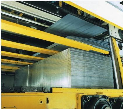
Uninterrupted destacking feature: forks (upper left) support the remaining blanks while the next stack is positioned on the lift table underneath.
