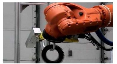
Robotically loading the front of a machine without a centering or gage station with accuracy unequalled by conventional automation because the robot knows exactly where the part is at all times.
