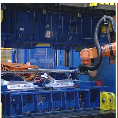
Robotic automation between tandem presses may not be the fastest solution, however for certain applications they provide the flexibility required. These applications may include an extremely large or heavy blank, the need for precise placement in the press or the requirement to turn a blank over.
